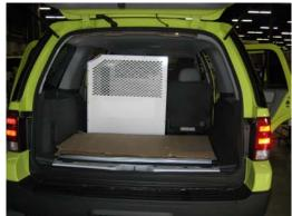
Slide K9 section of assembly through back hatch of vehicle. *Be careful npf4tp\_rip\_headlinger or scratch trim panels.*
